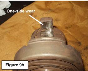
NOTE: Only use Optimol Olista Longtime 3EP VH 660865517 to lubricate the clutch release fork assembly.
